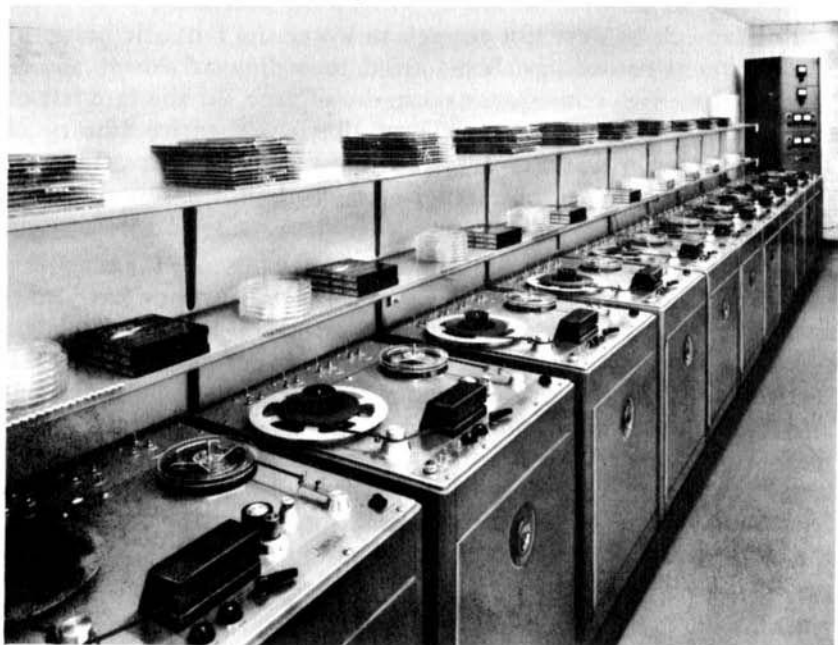
Fig. 405. Duplication of tapes for commercial release is cumbersome and time-consuming, resulting in high retail prices. The master unit at the far right feeds a maximum of ten "slave" recorders, running at 60 ips, and takes four minutes to duplicate a standard 1200-foot reel of tape. (Ampex)
